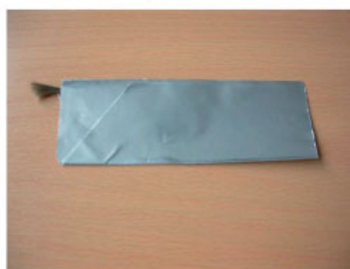
Each aluminium foil is to be folded once as shown above.
