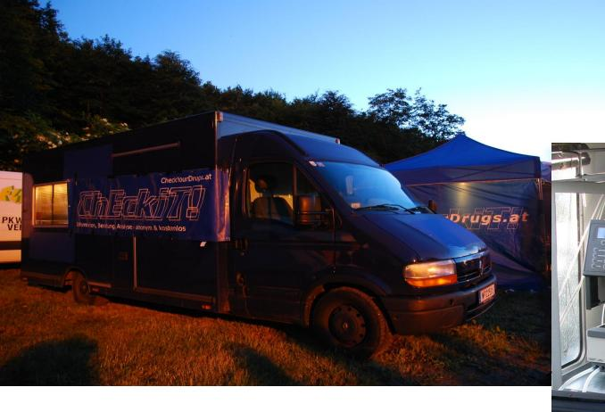
The mobile drug testing lab: using 4 HPLC systems and a LCMS system running in parallel for fast results.
